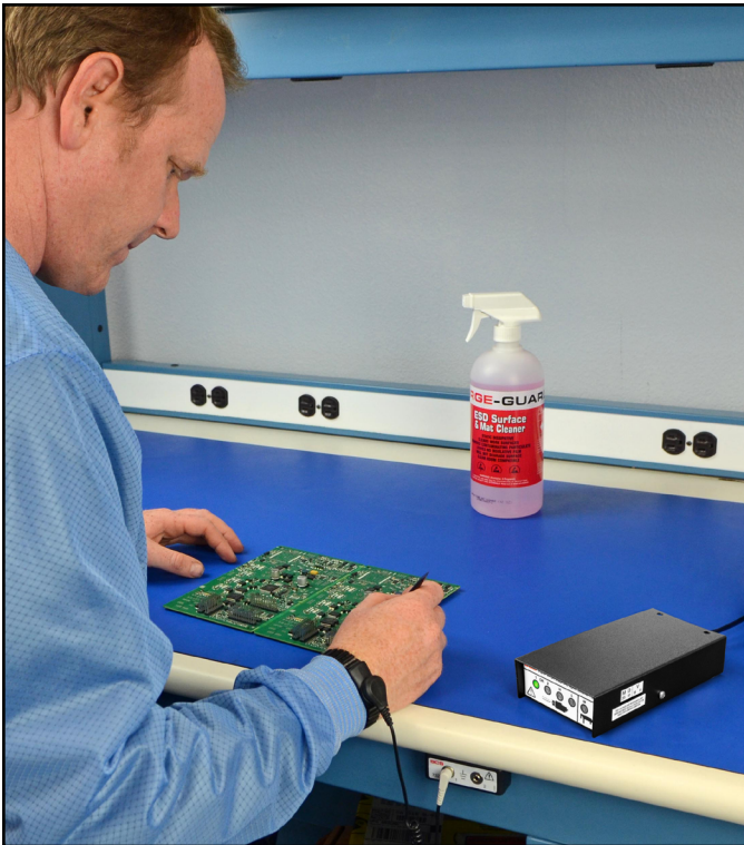
Figure 8. Using the 724 Workstation Monitor
