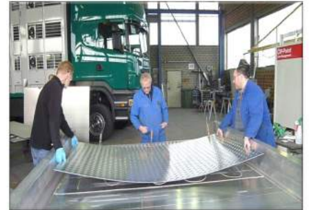
Figure 4: Next-Generation acrylic adhesives are an ideal replacement for welding and riveting joining methods in automotive, truck/trailer and enclosure applications.
