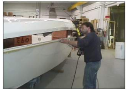
Figure 5: Next-Generation acrylic adhesives are useful in joining applications, such as recreational/marine, signs and facades, where mechanical fastening may not be possible or practical.
