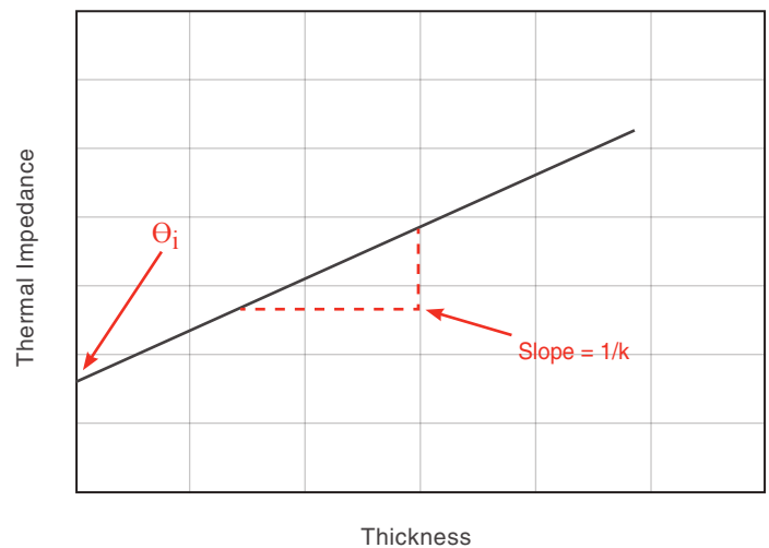
Figure 3: Determination of bulk thermal conductivity, k , (inverse slope) and thermal interfacial impedance, \theta_i , (y-intercept) from thermal impedance versus thickness measurements
