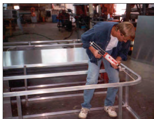
Figure 2: Using a handheld cartridge, a worker easily applies adhesive during sign assembly
